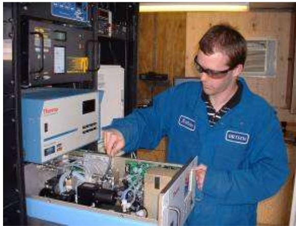
*An Ortech Environmental field consultant services a sulphur dioxide air quality monitor at an SLEA's monitoring station, as part of an ongoing instrumentation maintenance program. Reliable service and accurate data are hallmarks of the association's monitoring network.*
