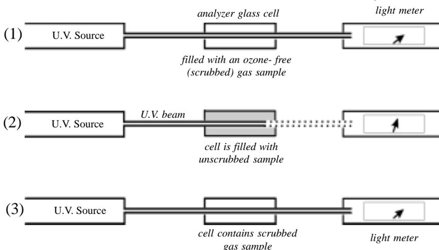
*Light intensities of steps (1) and (3) are averaged to obtain a reference standard or zero. When the intensity of light transmitted in (2) is compared with the reference/zero, the ozone concentration in the sample can then be determined.*
