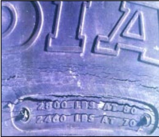
Ozone produces surface cracks on some molded rubber products. The severity of such attacks depends on the ozone concentration and also on the stress (tension) on the tire.
