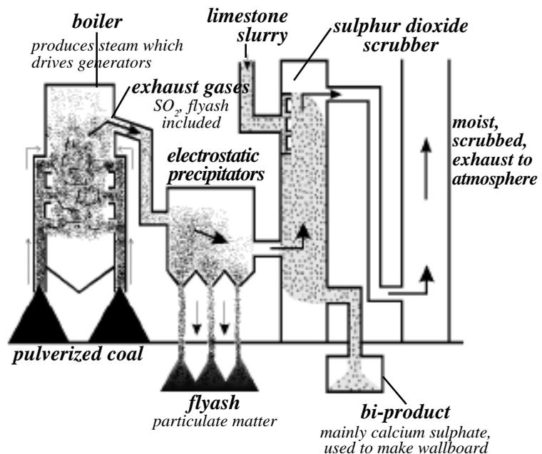
**Electrostatic precipitators** remove 99% of the flyash from waste gas streams by imparting negative charges to particles in the gas stream; the particles are then attracted to positive collecting plates. Periodic rapping of the collecting plates removes the particles.
