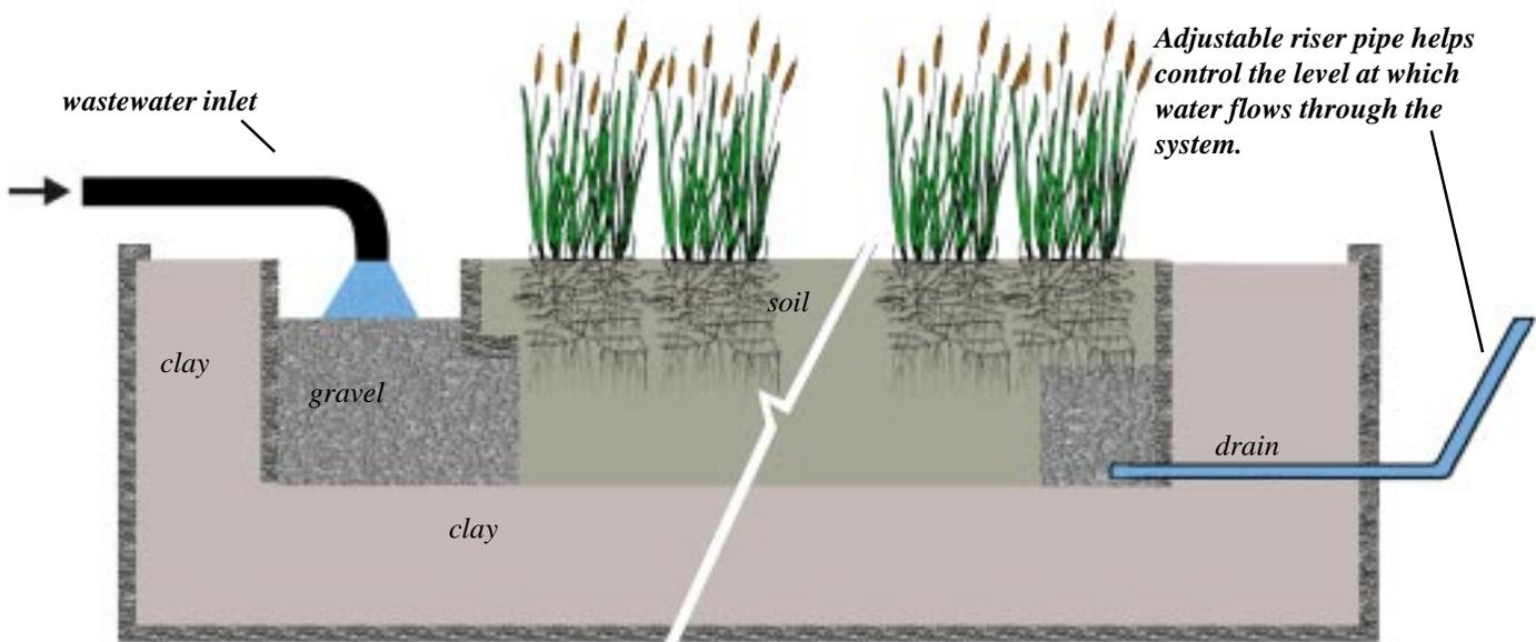
Microbes that treat the wastewater live on the gravel, soil and plant surfaces; the plants provide oxygen and food for the microbes. The removal of pollutants in wetlands is done mainly by microbes.
