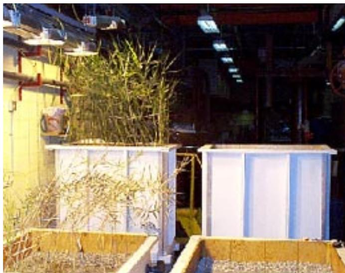
The two wetland systems pictured are subsurface flow types, ie. water levels are maintained below the surface of the soil. Each of these two systems contains a vertical subsurface flow unit as well as one that is horizontal, one system contains plants, the other is unplanted. The purpose of this difference, is to determine the extent to which plants assist in removing contaminants.
