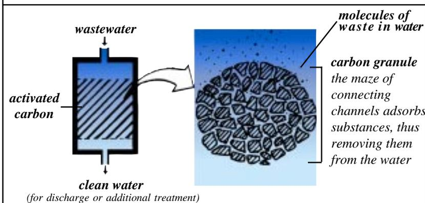
Activated carbons are highly porous; they contain mazes of interconnecting channels. **An imbalance of molecular forces in the walls attracts many substances; these are physically held (adsorbed) by the carbon surfaces.** After much use, the carbon may be re-generated and used again.
